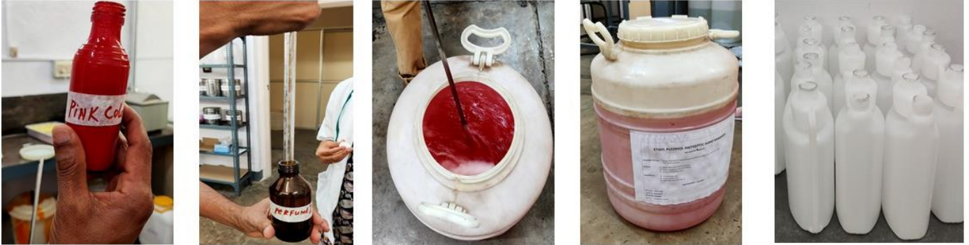
Step 4: Adding 10 ml of perfume and colouring agent to the solution and mixing it using a spatula and distributing in 1000ml bottles
